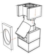
**FINISHING THE CHIMNEY:** Cut the insulation at the same level the casing block finishes. Next, put on the top plate and set the liner cutting line with a provision of ~1" ventilation gap. Cut the liner accordingly. Then install the clay pot adaptor in order to provide a base for the pot and glue the pot to the adaptor.
