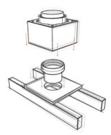
**CLEANOUT:** Cut out the afore-marked parts of the casing blocks. Measure and cut out pieces of insulation to make room for the cleanout branch.
