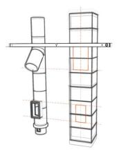
**SIDE INSTALLATION BASE:** Measure and cut out a hole for the ventilation grille in the first casing block from the bottom.
