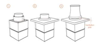
**GLUE MIXING & APPLICATION:** Mix boot ceramic and casing block glue according to the instructions on the packaging.
