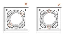
**REINFORCEMENT RODS:** When installing reinforcement rods it is good to have at least two pairs overlapping on different levels. Alternatively each rod may be on a different level.
