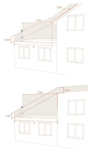
at least 2,3m from a structure and not less than 0,6m above the line connecting the extension edge or 10m (whichever longer) and the higher roof edge (also including separate buildings).
