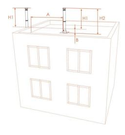
on a completely flat roof with no projections or if A is over 10 x B, H2 has to be minimum 250mm. In case there are projections on the roof then: A < 1,5m, H1 has to be minimum 0,6m A > 1,5m, H2 has to be minimum 0,6m If roof projections are complex please refer to BS 5440: Part 1, Section 4.
