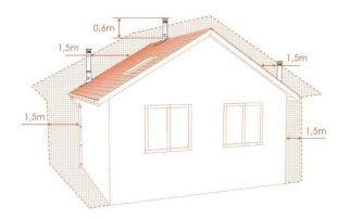
at least 1,5m measured horizontally from the wall or the roof surface or at least 0,6m over the roof ridge.
