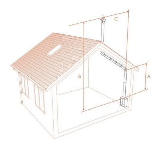
B should be at least twice as big as C and needs to be in accordance with either BS EN 13384-1/2 or equivalent height data in BS 5440 Part 1.
